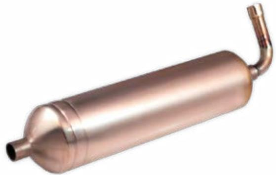
Applicable for household air conditioner compressor, the Accumulator is installed in front of the compressor to separate refrigerant and refrigeration oil and impurities not completely gasified by evaporators. It has functions of gas-liquid separation, liquid storage, oil return and noise reduction to ensure that the compressor would not be damaged by fluid impact.
